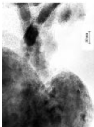
Fig. 4 High resolution electron microscopic image of \alpha\text{-Fe}^0 obtained from the decomposition of hexacetyl-bis(dimethylsulfoxide)-tri-iron(II), \text{Fe}_3(\text{CH}_3\text{COO})_6(\text{DMSO})_2 , in a 5% \text{H}_2/95\% Ar atmosphere obtained above 450^\circ\text{C}
